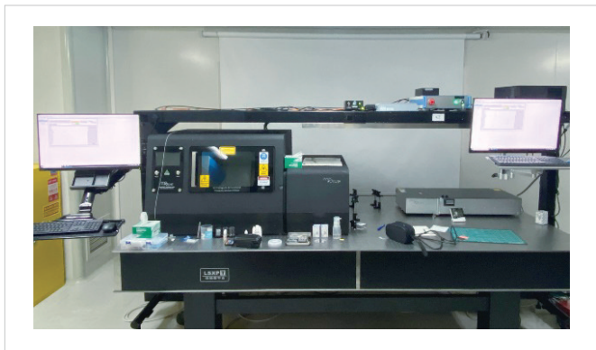
▲ Figure 3. Picture of femtosecond laser process system
